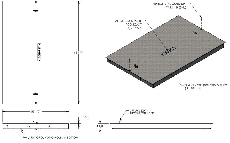
**NOTE 1:** FOR ADDED SECURITY, PENTA HEAD (P/N: PTA.38-1.5) OR SURELOCK BOLTS (P/N: SL.38-1.25) CAN BE ADDED **NOTE 2:** TREAD ON DIAMOND PLATE ADDS 1/8" TO OVERALL HEIGHT
