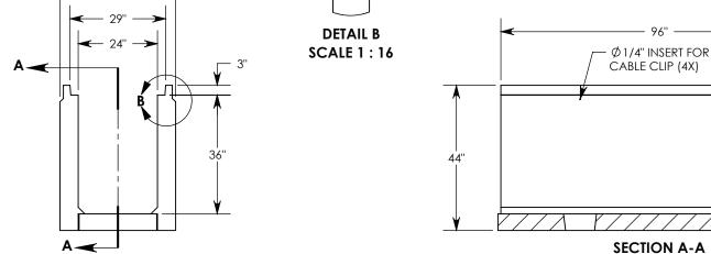
**NOTE 1:** FOR NON-STANDARD LENGTHS, THE CHANNEL WILL BE SOLID BOTTOM AND DESIGNATED WITH ITS CORRESPONDING LENGTH MEASUREMENT. IE: 802436HT3 32"
