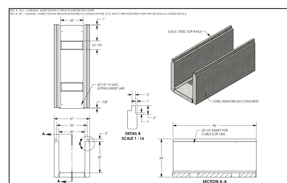
**NOTE 1:** FOR NON-STANDARD LENGTHS, THE CHANNEL WILL BE SOLID BOTTOM AND DESIGNATED WITH ITS CORRESPONDING LENGTH MEASUREMENT. IE: 803036HT3 32"
