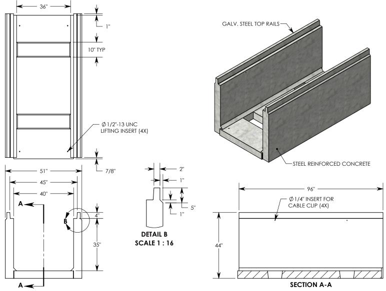
**NOTE 1:** FOR NON-STANDARD LENGTHS, THE CHANNEL WILL BE SOLID BOTTOM AND DESIGNATED WITH ITS CORRESPONDING LENGTH MEASUREMENT. IE: 804036HT4 32"
