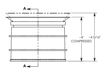
$\phi$  4 5/8" Ø4 1/8" 3 7/16" KNOCKOUT-− Ø41/2" · **SECTION A-A SEAL RING HIDDEN**
