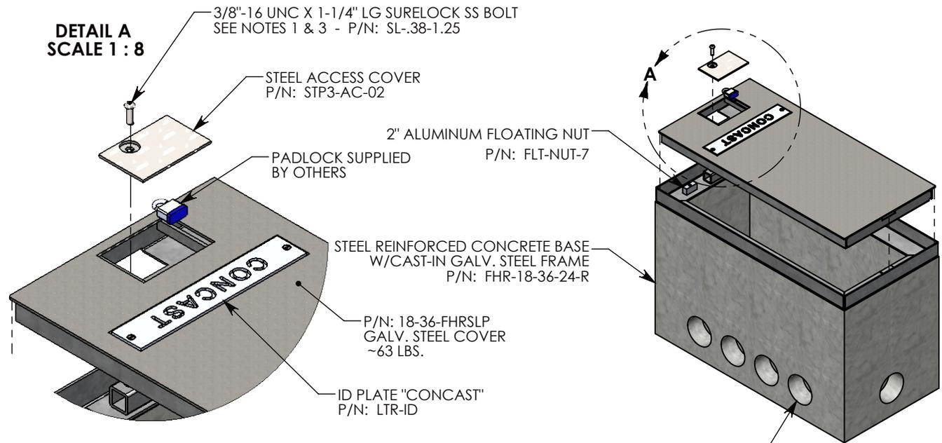
CON-DUCT TERMINATIONS ARE CAST INTO BOX SIDEWALLS. THEY FIT UP TO 4" PVC PIPE. TO ACCESS THE HOLES, BREAK PLASTIC SEAL. SEE NOTE 2.
