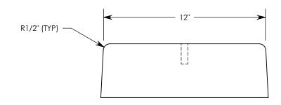
7,500 PSI CONCRETE UNLESS OTHERWISE DIRECTED, THIS PAD IS SUPPLIED AS SHOWN WITH NO CABLE ROUTING OPENINGS. IF OPENINGS ARE REQUIRED, MARK UP THIS DRAWING WITH THEIR LOCATIONS AND SIZES.
