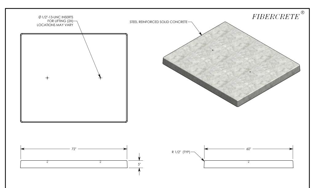
7,500 PSI CONCRETE UNLESS OTHERWISE DIRECTED, THIS PAD IS SUPPLIED AS SHOWN WITH NO CABLE ROUTING OPENINGS. IF OPENINGS ARE REQUIRED, MARK UP THIS DRAWING WITH THEIR LOCATIONS AND SIZES.
