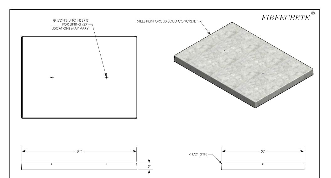
7,500 PSI CONCRETE UNLESS OTHERWISE DIRECTED, THIS PAD IS SUPPLIED AS SHOWN WITH NO CABLE ROUTING OPENINGS.
