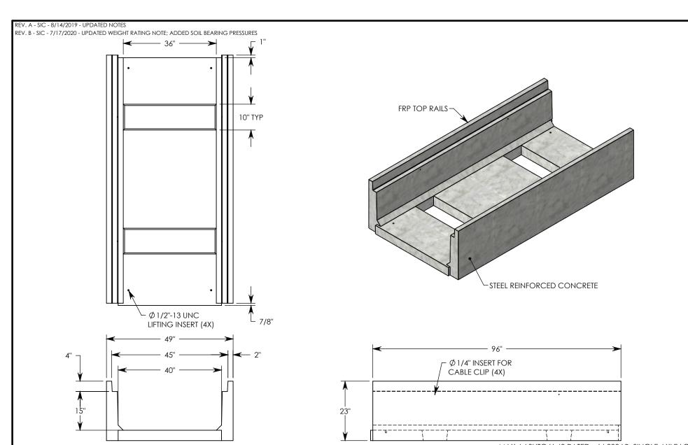
**NOTE 1:** FOR NON-STANDARD LENGTHS THE CHANNEL WILL BE SOLID BOTTOM AND DESIGNATED WITH ITS CORRESPONDING LENGTH MEASUREMENT. IE: HT4F4016 72"
