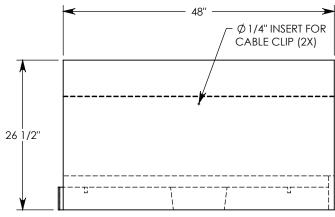
**NOTE 1:** FOR NON-STANDARD LENGTHS THE CHANNEL WILL BE SOLID BOTTOM AND DESIGNATED WITH ITS CORRESPONDING LENGTH MEASUREMENT. IE: HT6F2416 32"
