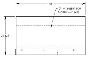
**NOTE 1:** FOR NON-STANDARD LENGTHS THE CHANNEL WILL BE SOLID BOTTOM AND DESIGNATED WITH ITS CORRESPONDING LENGTH MEASUREMENT. IE: HT6F3016 32"
