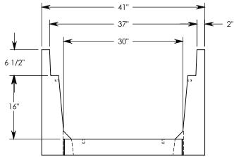
FRP TOP RAILS STEEL REINFORCED CONCRETE
