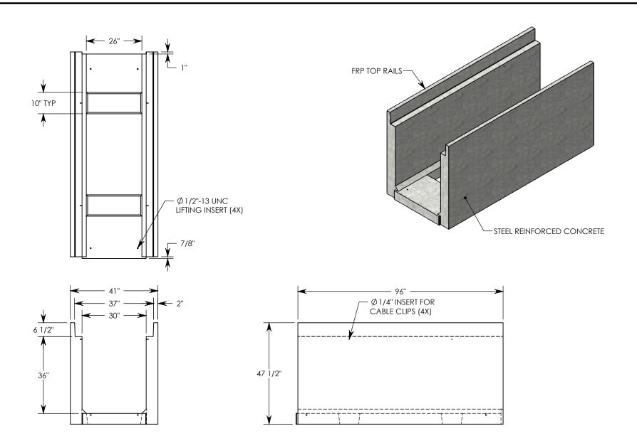
**NOTE 1:** FOR NON-STANDARD LENGTHS THE CHANNEL WILL BE SOLID BOTTOM AND DESIGNATED WITH ITS CORRESPONDING LENGTH MEASUREMENT. IE: HT6F3036 36"
