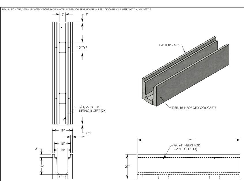
**NOTE 1:** FOR NON-STANDARD LENGTHS THE CHANNEL WILL BE SOLID BOTTOM AND DESIGNATED WITH ITS CORRESPONDING LENGTH MEASUREMENT. IE: HTF1016 32"
