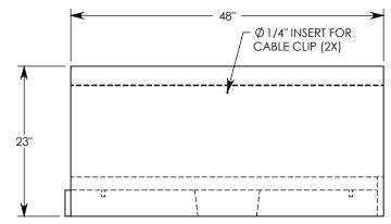
**NOTE 1:** FOR NON-STANDARD LENGTHS THE CHANNEL WILL BE SOLID BOTTOM AND DESIGNATED WITH ITS CORRESPONDING LENGTH MEASUREMENT. IE: HTF2416 32"
