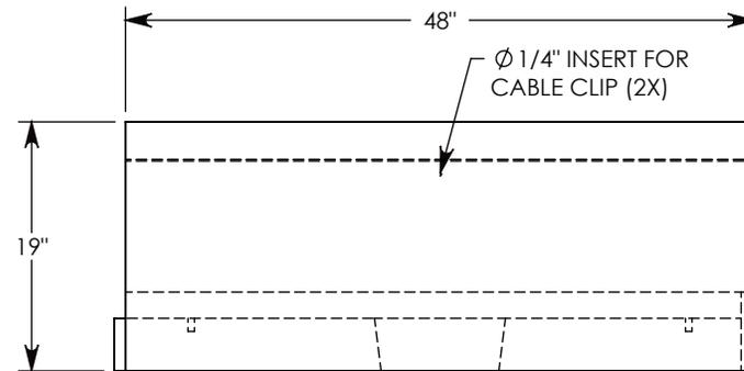
**NOTE 1:** FOR NON-STANDARD LENGTHS, THE CHANNEL WILL BE SOLID BOTTOM AND DESIGNATED WITH ITS CORRESPONDING LENGTH MEASUREMENT. IE: HTF4012 32"
