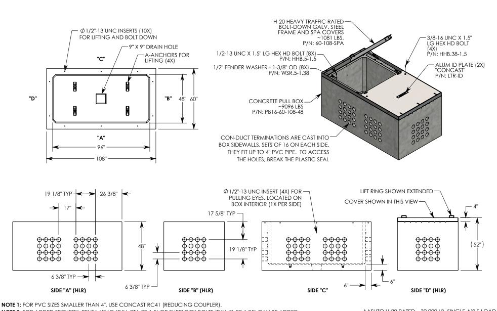
NOTE 2: FOR ADDED SECURITY, PENTA HEAD (P/N: PTA.38-1.5) OR SURELOCK BOLTS (P/N: SL.38-1.25) CAN BE ADDED
