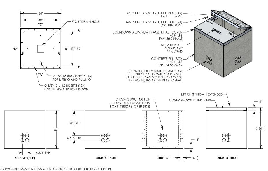
NOTE 1: FOR PVC SIZES SMALLER THAN 4", USE CONCAST RC41 (REDUCING COUPLER).
