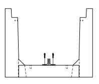
CLEAR DEBRIS FROM HOLES AND HAMMER ANCHOR PIN BOLTS (APB25-1.25) INTO DRILLED HOLES
