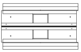
DRILL HOLES THROUGH THE DIVIDER BASE AND INTO THE CHANNEL A MASONRY BIT IS RECOMMENDED
