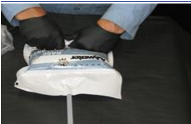
Bursting secondary seal
