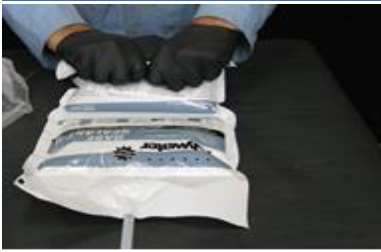
Burst primary seal
